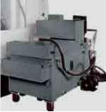
Belt filter unit on cooling water tank
