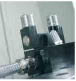
Laser tool measuring device
