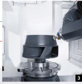
1: Machining a diffuser case from Inconel 718 with an ULTRASONIC 125 FD 2: ULTRASONIC 60 FD duoBLOCK:
