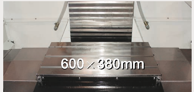
The largest table size in its class and the perfect slide way construction, which blocks all chips and coolant that might stream down into the inner side of slide way.
